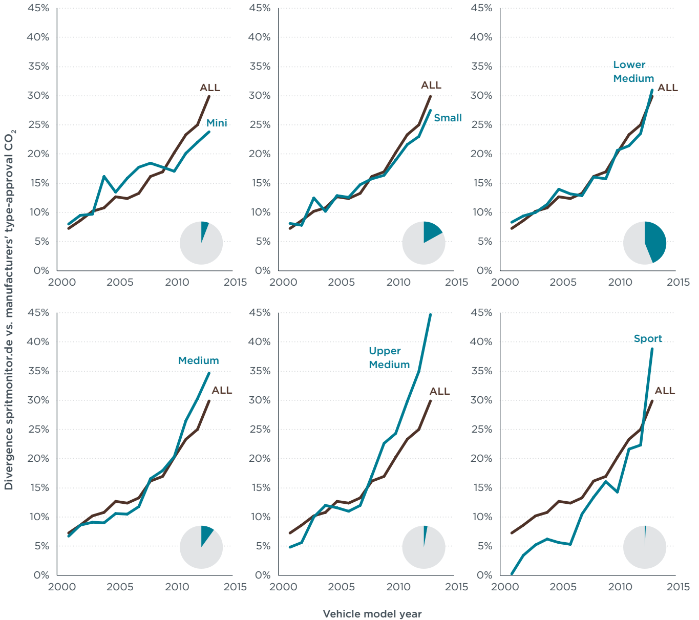
Figure 5. Divergence of spritmonitor.de vs. manufacturers' type-approval values by vehicle segment (pie chart indicates number of vehicles per segment in the data set for 2013).
