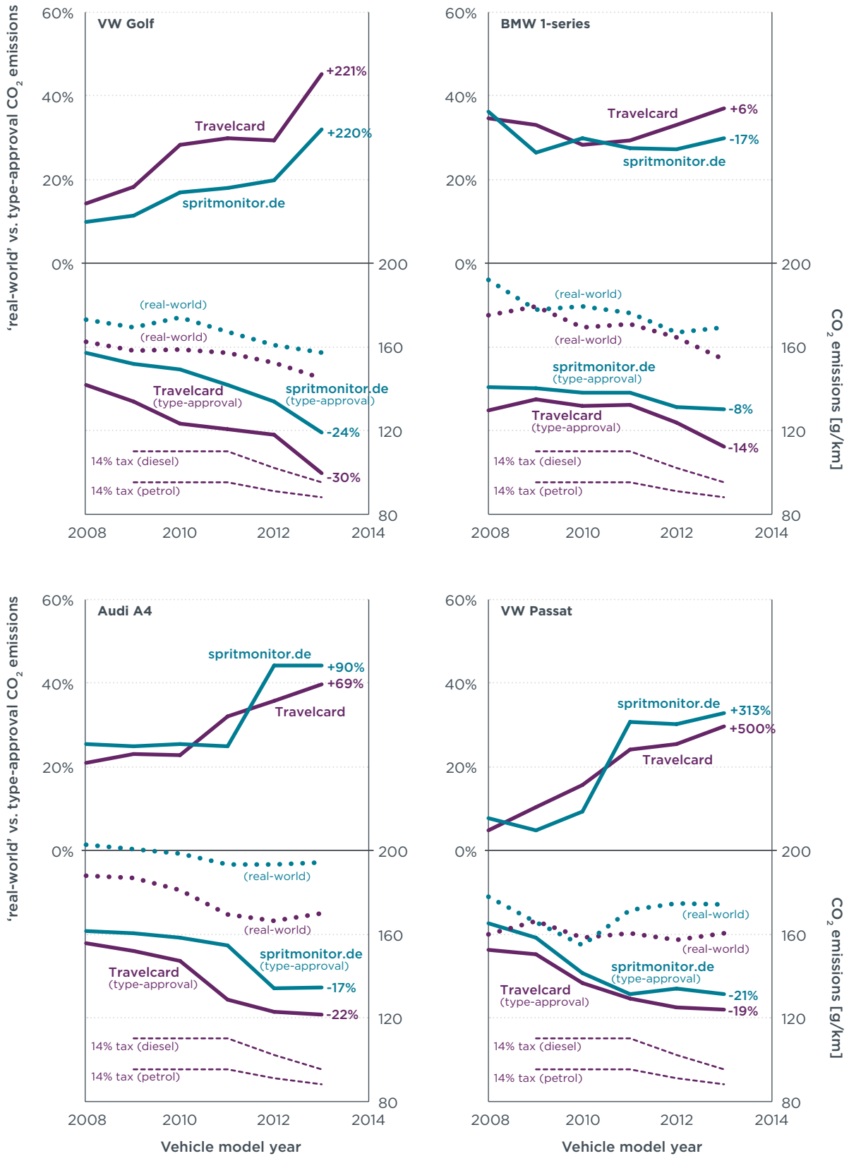
Figure 26. Comparison of spritmonitor.de and Travelcard data by vehicle model (models outside the Netherlands' 14 percent tax threshold).
